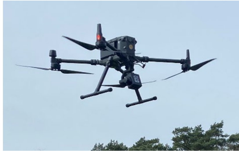
The BlackBird V2 from HAIP manufacturer, mounted on the Matrice M300
