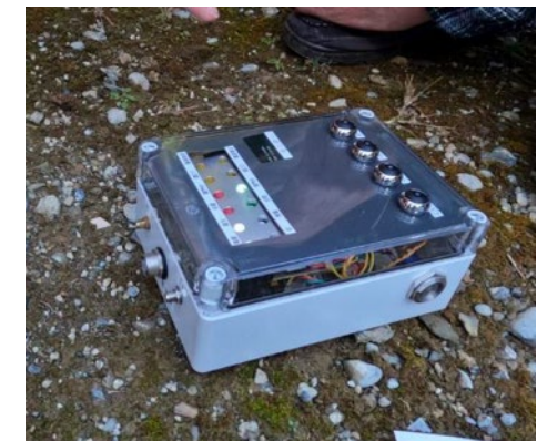
Remote controller of water gate opening/closing
