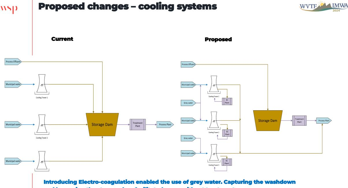
and bypassing the storage dam facilitated reuse without treatment.
