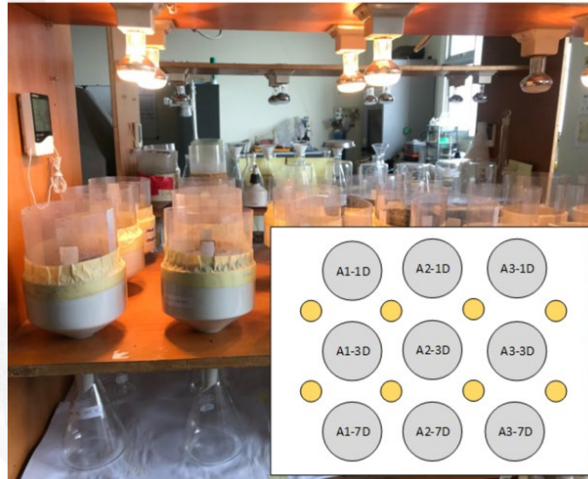
Schematic of Kinetic Test in the Laboratory using FDCLT method and Various Wet-Dry Cycle
