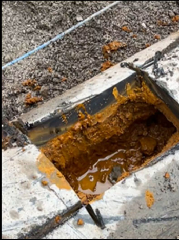
Iron Scale In Pressurized Line
