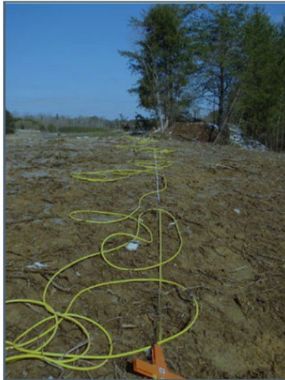
Figure 2. ERT setup on Line 3 SVC Site, Dunlap, TN
