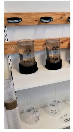
40 weeks with weekly cycles of water saturation and air drying
