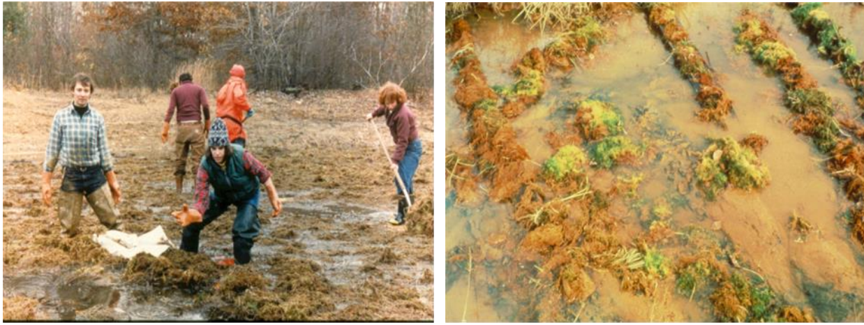
Figure 2A. Attempted recreation of a sphagnum moss bog at the Friendship Hill site by USBM staff; photo shows young versions of Bob Hedin, Michelle Girts, and Trish Erickson. B. Eventual result: the high iron concentrations at the site slowly overwhelmed the moss's adsorptive capacity.
