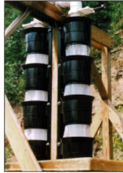
Water is oxygenated before flowing into the fish tanks by a simple mechanical means of exposing to to fresh air.
