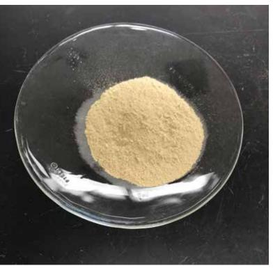
Figure 4. West Virginia University's REE Extraction Facility produces highly concentrated rate earth products from AMD precipitates. This sample is 87 percent rare earth oxide.
