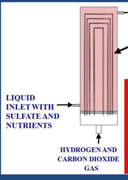
SULFATE 71 MICROPOROUS, HOLLOW FIBER WITH BIOFILMS OFACTIVE SRB No gas recycle No gas separation of H<sub>2</sub>S **Biofilm instead of suspended** (Minimal washout; Critical due to low biomass yield) Excellent mass transfer Compact 5.0
