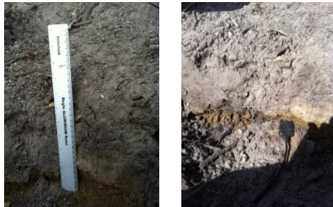
Reconstructed soil profile with water potential sensors
