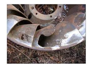
In most cases, cavitation is an undesirable occurrence. In devices such as propellers and pumps, it causes vibration, noise, loss of efficiency and damage to components.
