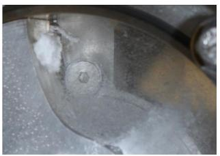
High speed photography (1000 fps) shows the powerful rolling harnessed cavitation field generated within the reactor core. While it is a destructive force, this cavitation does not affect the reactor itself in any way.
