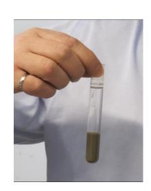
Recovered 2.5 L of Bitumen from 60 L of Tailings
