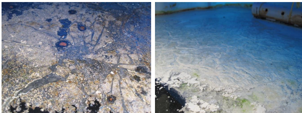
Figure 5. Precipitates on the water surface of mussel shell reactors.
