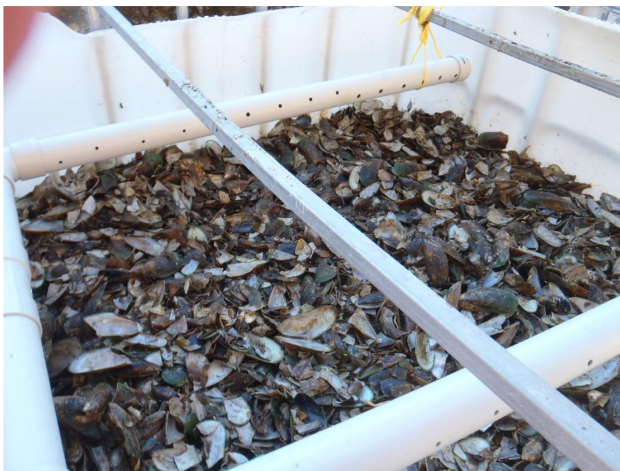
Figure 1. Mussel shells in completed mussel shell reactor prior to filling with water.
