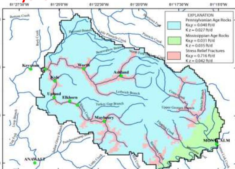
Figure 8. Distribution of hydraulic conductivity in layer 3 of the numerical groundwater flow model developed for the Elkhorn area, McDowell County, West Virginia.
