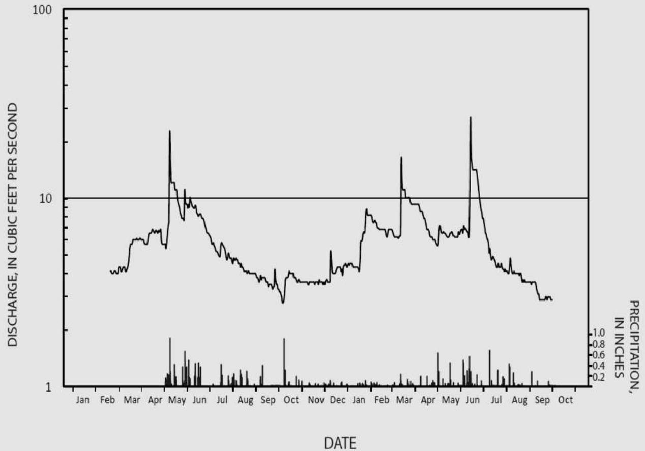
Figure xx. Hydrograph and precipitation from USGS gaging station 03212640 Johns Knob Branch at Elkhorn, West Virginia.
