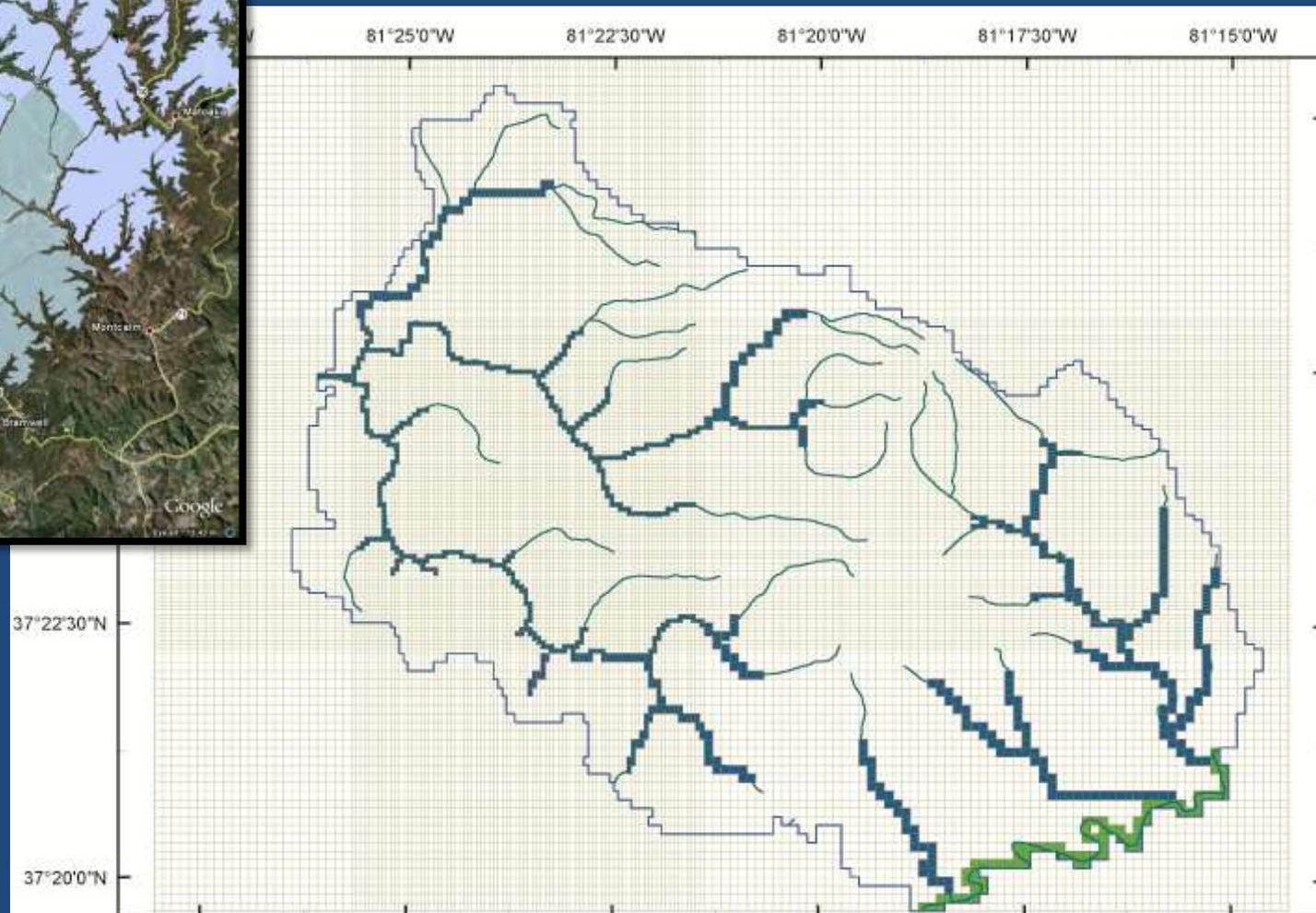
Figure #. Map showing the domain, drain cells simulating streams, river cells, no-flow boundaries, and the finite difference grid for the numerical groundwater-flow model developed for the Elkhorn area, McDowell County, West Virginia.
