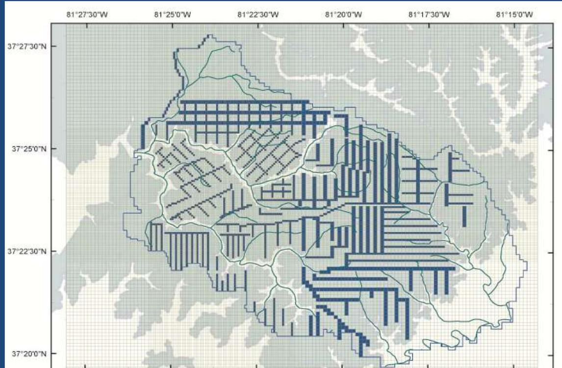
Figure #. Locations of drain cells used in the numerical groundwater flow model to simulate the free-flowing mine entires of the abandoned Pocahontas No. 3 coal mine workings in the Elkhorn area, McDowell County, West Virginia.
