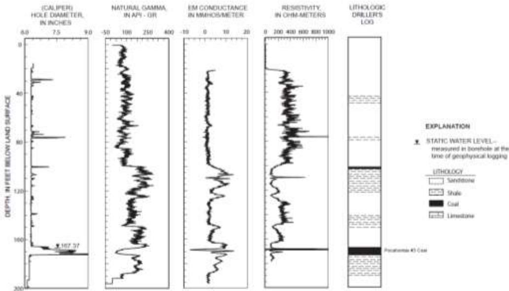
Figure XX. Borehole-geophysical logs for borehole Mcd-0205 (Well 7), collected on August 23, 2009, near Elkhorn, West Virginia.
