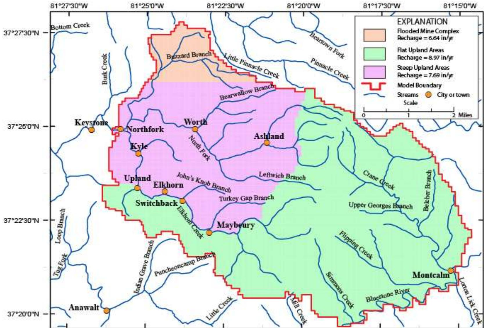
Figure 26. Recharge for three distinct regions within the numerical groundwater-flow model developed for the Elkhorn area, McDowell County, West Virginia.
