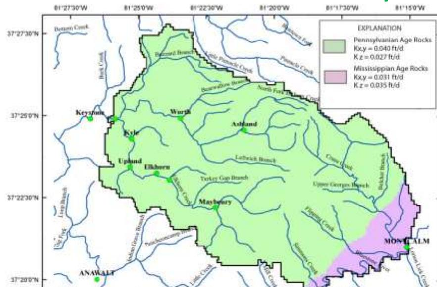
Figure 8. Distribution of hydraulic conductivity in layer 4 of the numerical groundwater flow model developed for the Elkhorn area, McDowell County, West Virginia.
