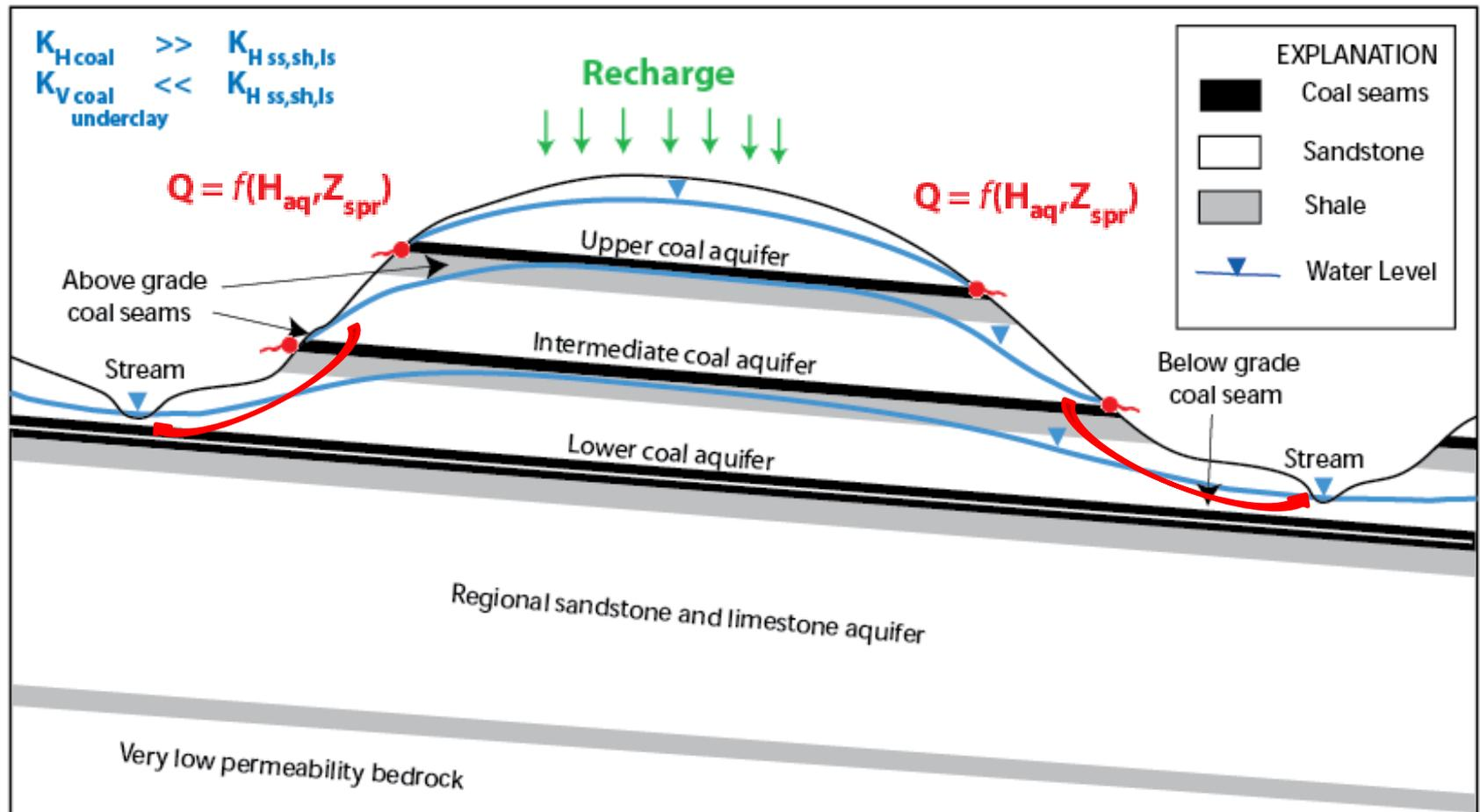
Figure \_\_\_\_ Conceptual model of perched aquifers in an unmined setting typical of the southern West Virginia coal province.
