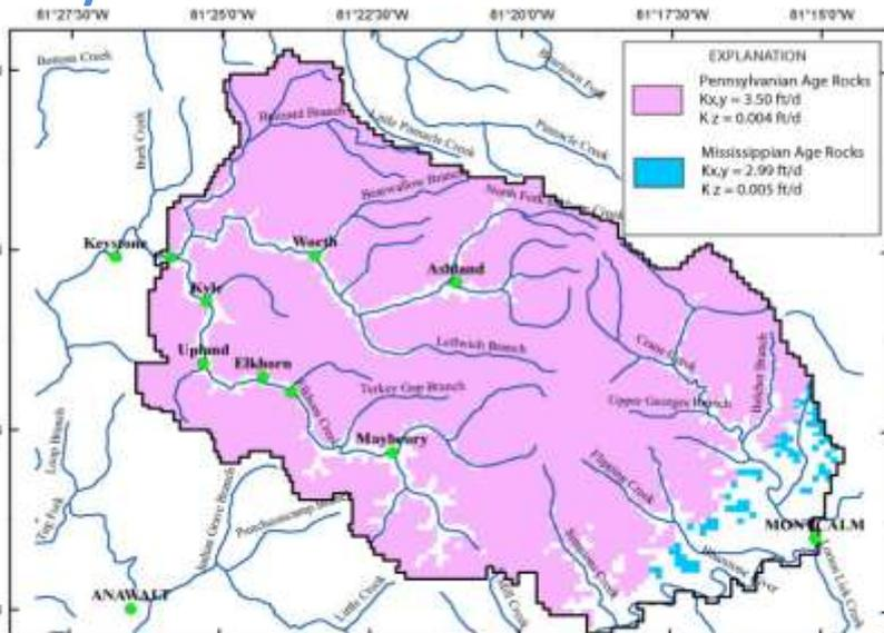
Figure 8. Distribution of hydraulic conductivity in layer 1 of the numerical groundwater flow model developed for the Elkhorn area, McDowell County, West Virginia.
