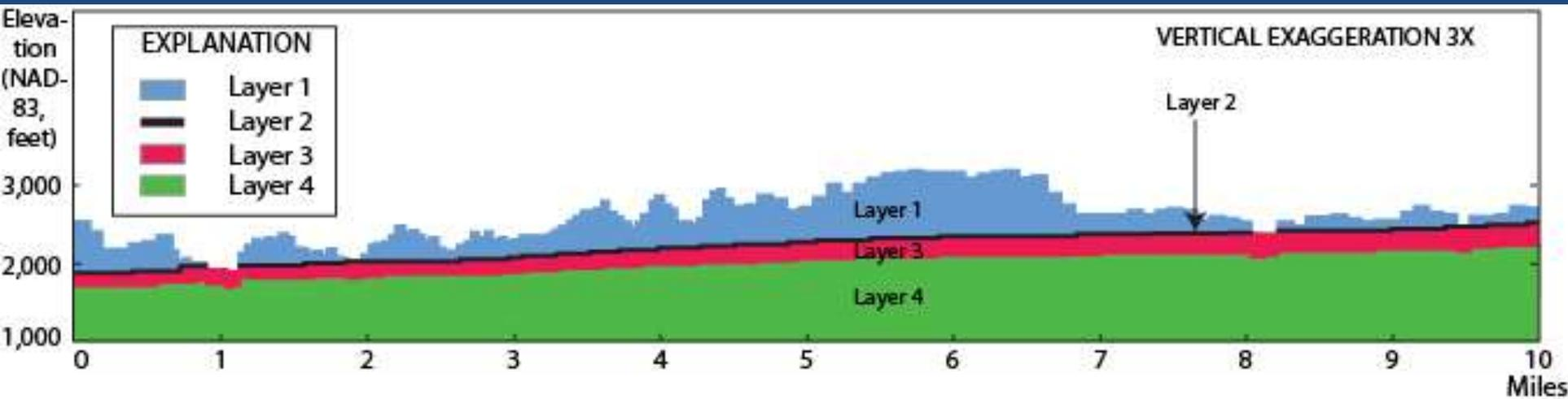
Figure 19. Cross section showing layers of the numerical groundwater-flow model developed for the Elkhorn area, Mcdowell County, West Virginia. [NAD-83, North American Vertical Datum of 1983; cross section patterned from row 89 of model].
