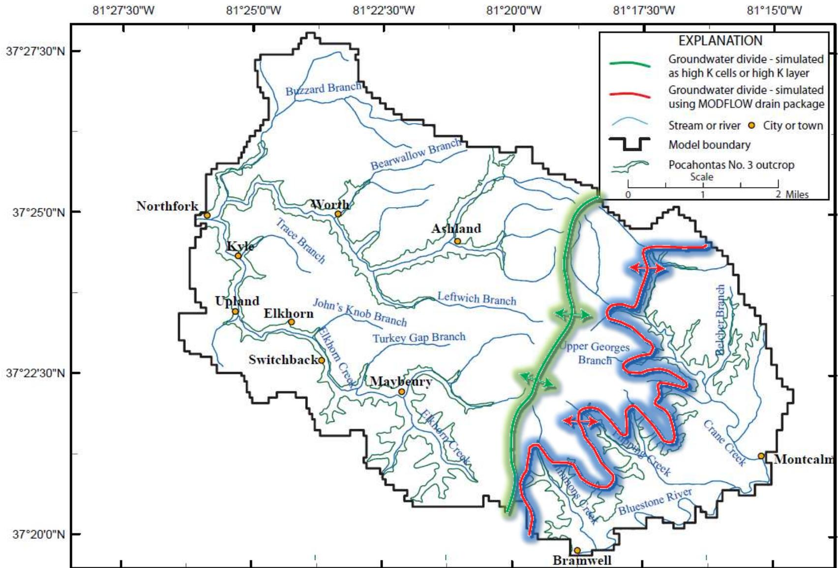
Figure \_\_. Approximate location of groundwater divides simulated either as A) high K cells in a low permeability matrix or as a high K layer, or B) simulated as drains in the groundwater-flow model for the Elkhorn area, McDowell County, West Virginia.
