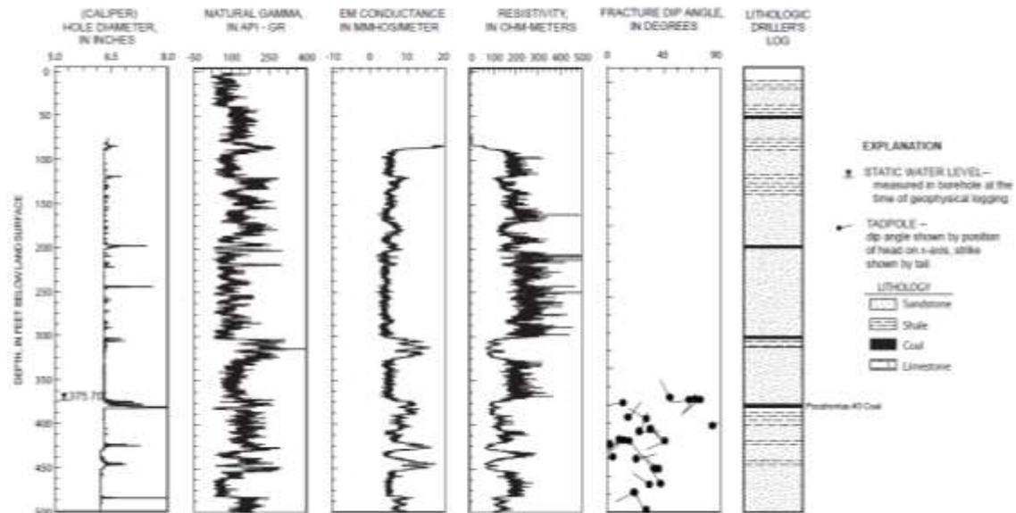
Figure XX. Borehole-geophysical logs for borehole Mcd-0205 (Well 5), collected on August 20, 2009, near Elkhorn, West Virginia.
