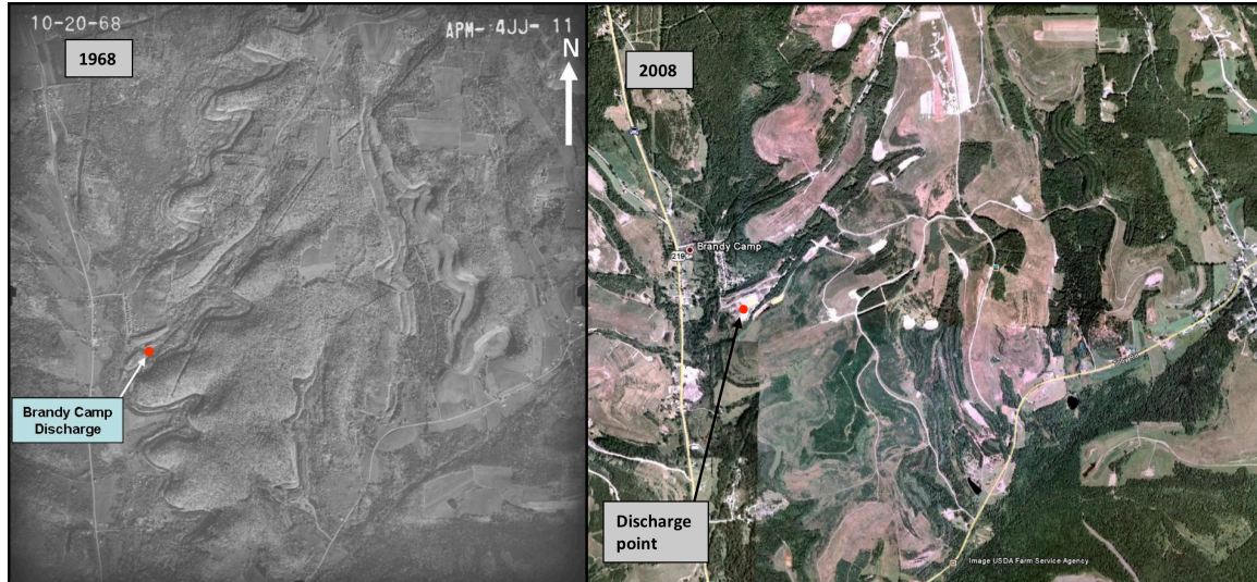
Figure 5. Aerial photograph from October 1968 (left) showing that much of the recharge area for the mines contributing to the Brandy Camp discharge was forested. Aerial photograph from May 2008 (right) showing mined areas.
