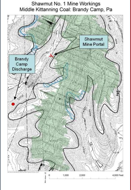
By opening up an old sealed portal we determined that a portion of the mine pool could decanted off and an upper limit to the pool level could be achieved by creating an overflow outlet.
