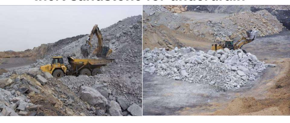
Most inert underdrain material located between the Lower Stockton seam and the Coalburg rider.
