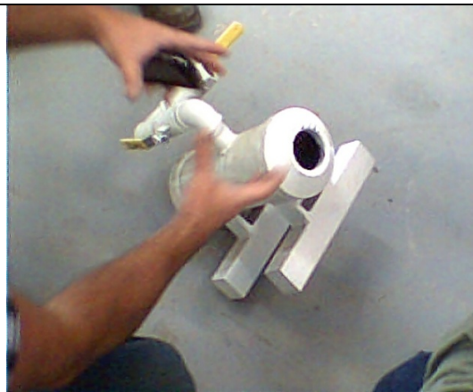
Figure 3. Static mixer used to combine solid and foam components to create pHoam TM
