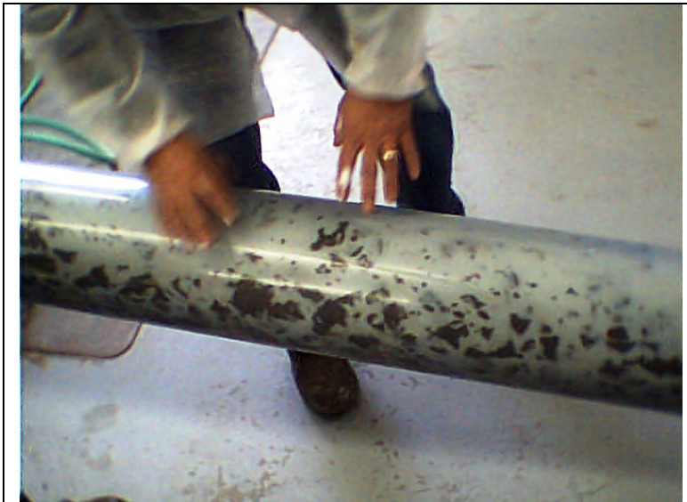
Figure 6. Gravel in column is encapsulated with pHoam TM after feed was suspended
