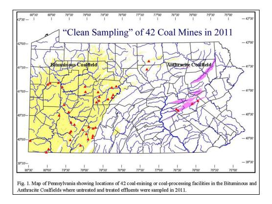
COAL MAP: Clean sampling and analysis procedures were used to quantify more than 70 inorganic chemical constituents, including 36 "priority pollutants," organic carbon and phenols, and other characteristics of untreated (influent) and treated (effluent) discharges at 38 permitted coal-mining or coal-processing facilities in the bituminous coalfield and 4 facilities in the anthracite coalfield of Pennsylvania.
