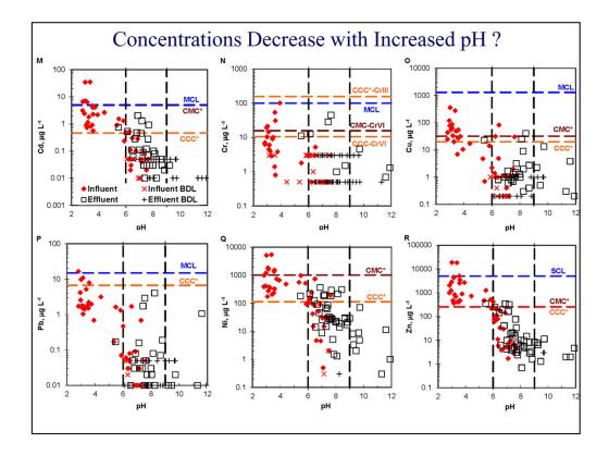
ENVIRONMENTAL SIGNIFICANCE: Without considering sample hardness, acidic samples (pH < 6) and some pH-compliant samples (pH  $\ge$  6) had elevated concentrations of Cd, Cr, Pb, Ni, and/or Zn compared to the aquatic CMC or CCC levels. However....
