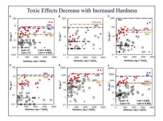
ENVIRONMENTAL SIGNIFICANCE: After correcting for sample hardness, all pH-compliant samples (pH  $\geq$  6) had concentrations of Cd, Cr, Pb, Ni, and Zn that were less than CMC levels. One pH-compliant sample exceeded the CMC value for Cu.
