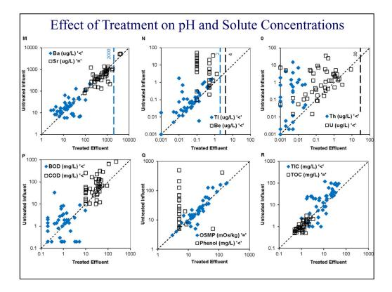
EFFECT OF TREATMENT: The Wilcoxon matched-pair signed-ranks test was used to test the hypothesis that the difference between the effluent and influent pairs was equal to zero. The tests computed the difference in composition between the effluent and the corresponding influent for each site. The absolute values of the differences for all the sites combined were rank transformed, and then the sign of the differences was reapplied to the ranks
