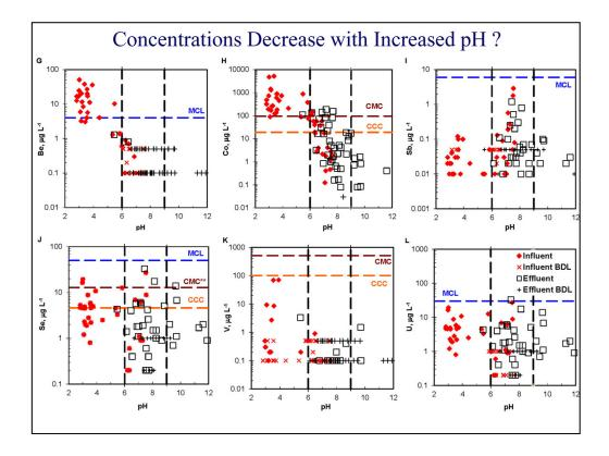
ENVIRONMENTAL SIGNIFICANCE: Permitted mine effluent must have pH 6 to 9. All but three effluents had net acidity concentrations greater than 0 (alkalinity > acidity) and pH ( $\geq$  6); some treated effluent had pH > 9. Although most of the treated effluents had greater than 250 mg/L SO4 threshold, only one sample had Fe greater than 7 mg/L. Several samples had Mn greater than 5 mg/L.
