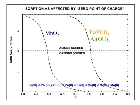
ADSORPTION: The adsorption of metals by Fe(III), Al, and Mn(IV) hydroxides accounts for the attenuation of most trace metals. Cations are adsorbed at high pH. Anions, such as SO4 and AsO3, are adsorbed at low pH.
