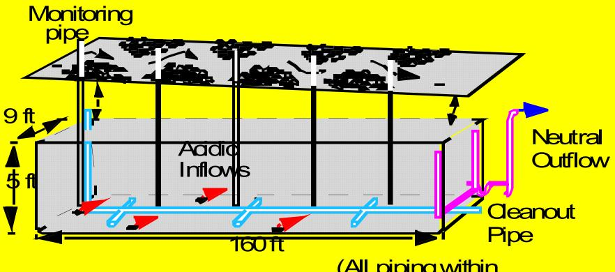
Limestone, 11/4-3 inch Limestone, <2 inch (All piping within drain is perforated)
