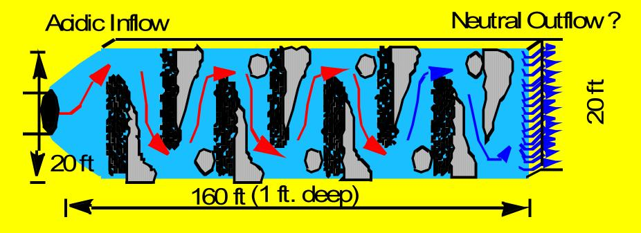
Limestone, 11/4 - 3 inch (66 tons) Limestone sand, < 1/2 inch (44 tons)
