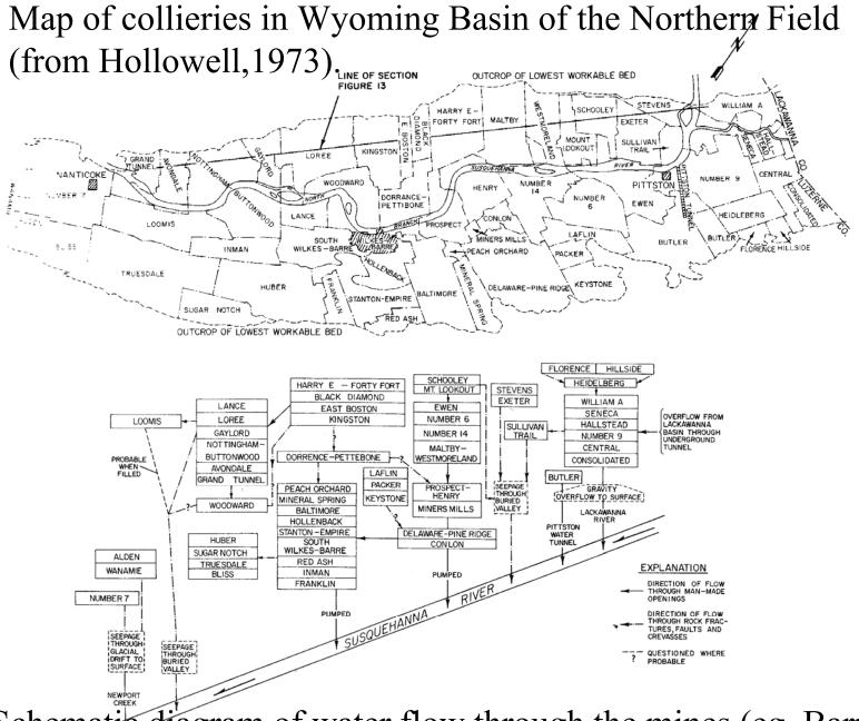
Schematic diagram of water flow through the mines (eg. Barrier pillar breaches) in the Wyoming Basin, (from Hollowell 1973).
