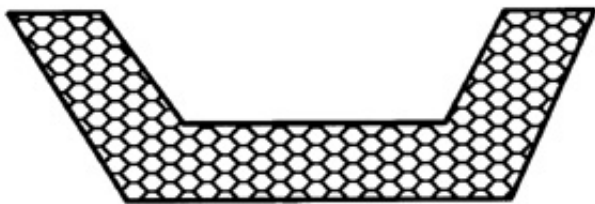
Figure 2 - Trapezoidal Open Limestone Channel
