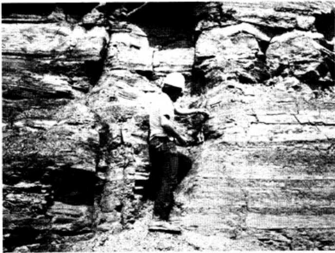
Figure 6: Sampling and analysis of overburden strata in the highwall are important in reconfirming premining overburden analysis or as new strata appear during mining.
