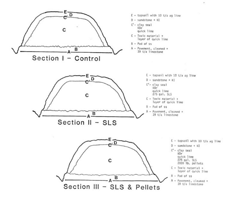
Figure 2 - Generalized Cross-Sections of the Three Areas of Prong Site Detailing Variations in C' Layer
